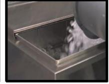
Fill the ice bin with clean ice. Note: The Ice Bin must be a minimum of 50% full for 20 minutes for proper dispensing temperature
