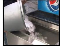
Fill the ice bin with clean ice. Note: The Fountain Ice Bin must be a minimum of 50% full for 20 minutes for proper dispensing temperature
